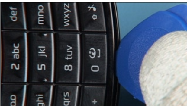
23. Carefully press at both edges, - like shown before. Lift out the BOTTOM KEYMAT SUPPORT.
